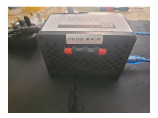
Additionally, we have replaced the fiddly screw terminals with push terminals, allowing for simplification and ease of use.
